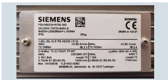
Fig. 12/4 Example, rating plate on the motor
